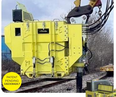
The 360-VAC® attachment converts your excavator into a wet and dry VAC-EX. Its multi-stage filtration system extends machine life and prevents dangerous exhaust dust.
